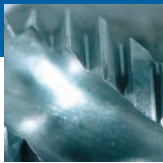
■ Cutting edge after 1.000 holes tapping
